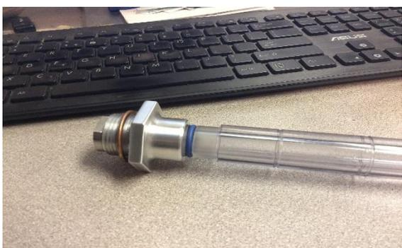
This shows the O-Ring seal installed at the top of the sight tube to create a positive seal.
