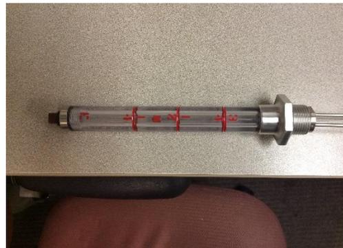
As can be seen in this picture the reinforcement ring at the bottom of the tube.
