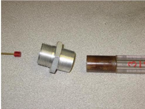
This is an example of what appears to be Shellac used to seal the sight tube to the retaining nut.
